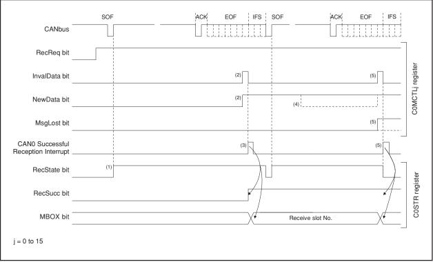
Figure 18.21 Timing of Receive Data Frame Sequence
